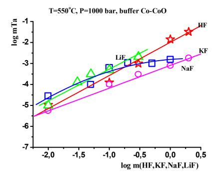
**Fig.1.** Concentration dependence of Ta<sub>2</sub>O<sub>5</sub> solubility at T=550° C, P=1000 bars in fluoride solutions HF, KF, NaF, LiF (Co-CoO buffer)
