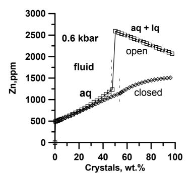
**Fig. 1.** Change of Zn concentration in fluid phase in the process of crystallization-assisted degassing of a rhyolitic melt at 0,6 kbar in the closed and opened conditions. The initial concentrations in the melt are:  $H_2O = 2.9$  wt. %, Cl = 0.15 wt. %, Zn = 100 ppm. For calculations it is accepted D(Zn)s/m = 0.6; D(Zn)lq/aq = 10. The vertical dashed lines show of beginning moment of heterogeneous fluid (aq+lq) exsolution from a melt.
