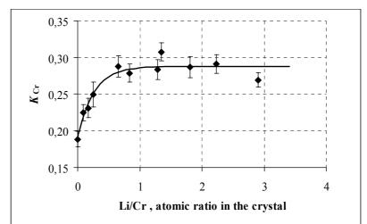
**Fig. 3.** Dependence of  $K_{Cr}$  from Li/Cr atomic ratio in the crystals
