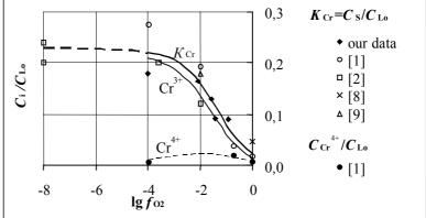
Fig.2. Dependence of  $K_{Cr}$  on  $f_{O2}$  and relation of different valent forms of chromium in the crystal All the points -the experimental data, all the curves - results of calculations.
