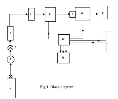
The setup incorporates the following: 1. Cylinder containing inert gas (Ar);
