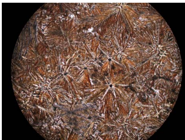
Variolitic texture of melanephelinite after experiment. View size is 1 mm. Parallel nicols.
