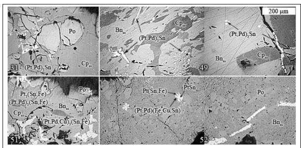
Fig. Pt-Pd-Sn alloys in associations with c chalcopyrite (Cpss), pyrrhotite (Po), and bornite (Bnss).
